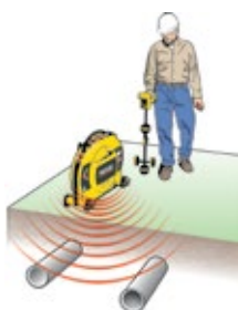
Induce a signal to locate utilities.
